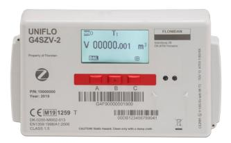
Symbols shown at the top of the display when either volume or balance screen is displayed.
